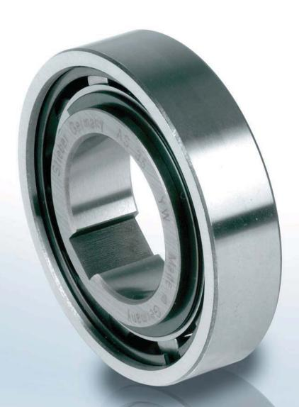
ype AS is a roller type freewheel non-bearing supported. Bearings are required to support axial and radial loads. Lubrication and sealing must also be provided by the installation. Nominal outside dimensions are the same as series 62.. ball bearings.
