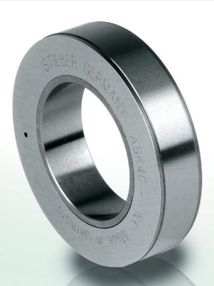
ype ASK is a roller type freewheel bearing supported by two rows of roller bearings. It is a self-contained dust protected unit, delivered grease lubricated.
