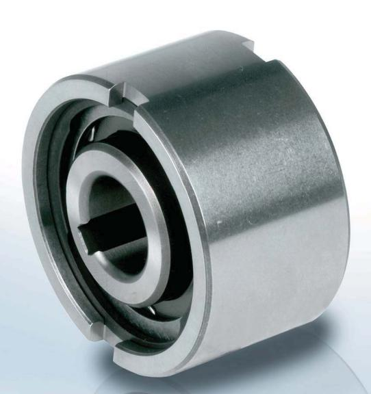
ype NF is a roller type freewheel non-bearing supported. Bearings are required to support axial and radial loads. Lubrication and sealing must also be provided by the installation.
