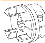
Type 2.3 Clamping hub with spline bore (For a selection of our programme of spline bores see page 36)
