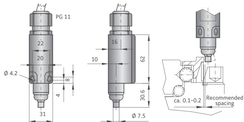
The switch plunger (pictured above and right) should be located as close to the actuation ring / limit switch plate as possible (approximately 0.1-0.2mm).
