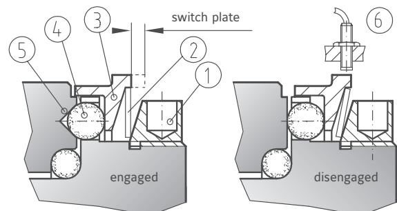
① Torque adjustment nut    ③ Switch plate    ⑤ Conical detent
